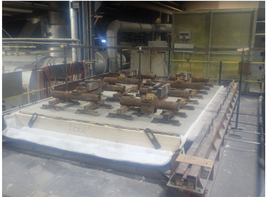
The unexposed face of the floor assembly after 10 minutes of testing
