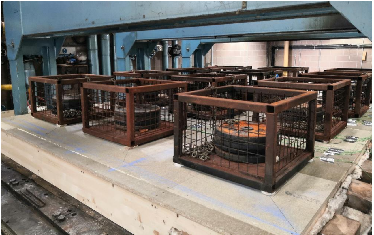
Photograph 8 - Overall view of the unexposed side of the sample, showing the position of the loading cages.
