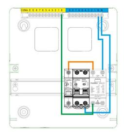
TAIL CLAMP (ACCF) CANNOT BE USED WHEN SPDCUKITT1 IS INSTALLED within a FuseBox consumer unit, unless an additional mounting hole is drilled by the installer for the clamp to be fixed.
