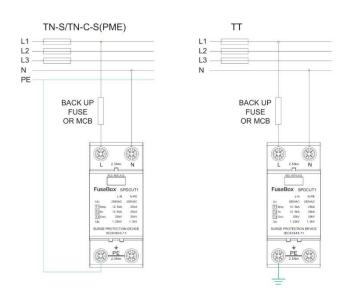
Before powering up the installation check all connections are TORQUED to 2.5Nm. Loose connections cause fires!
