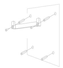
• Fix the hand dryer in place by hooking it into the bracket and securing it in place at the bottom using the fixings provided.
