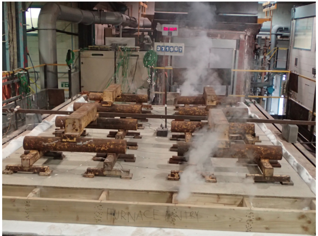
The unexposed face of the assembly after 36 minutes of testing
