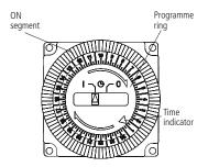
Time control segments: 1 seament = 15 minutes. push segment down for ON, pull up for OFF.
