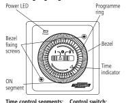
**Time control segments:** 1 segment = 15 minutes, push segment down for ON, pull up for OFF.
