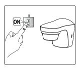
➤ Connect motion detector to power supply.
