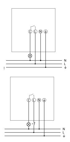
The device can be manually activated with a circuit breaker. After releasing the button (return of power) the device switches on (for at least 40 secs or for the time set on the device).
