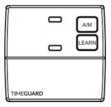
Press and hold the Learn button on the front of the receiver for 10 seconds until the blue Learn/Manual light starts flashing, the button surrounds will illuminate.  On the transmitter, press and hold both the + and Frost/Night Set-back buttons at the same time until the flashing blue Learn/Manual light goes off. This should take approximately 3 seconds.
